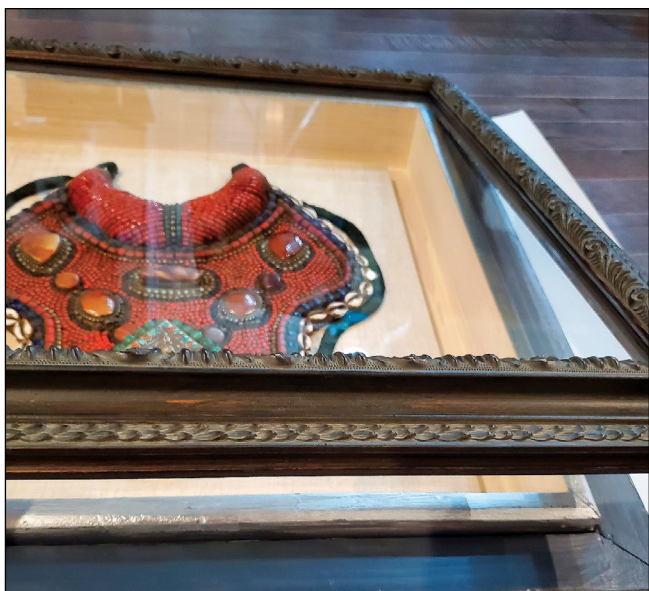
● A slip over the top frame allowed enough depth for the moulding and glazing to comfortably and securely fit over the base unit.
