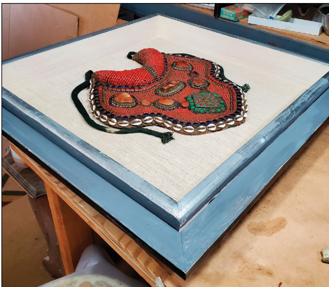
● Finished transition moulding attached to side of custom shadowbox by drilling finish screws through the sides.
